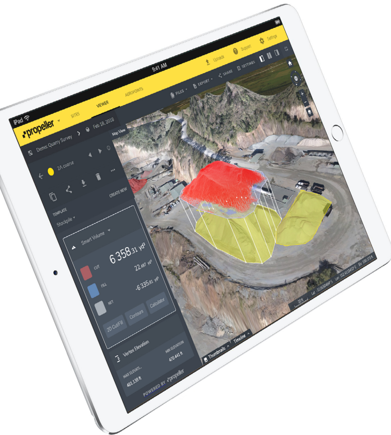
Quarry volume measured in 3D using drone photogrammetry software
